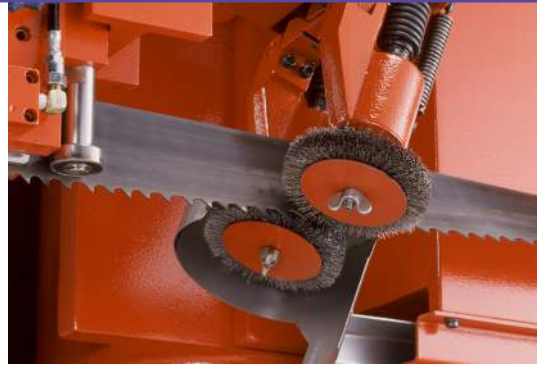
Automatic Dual Wire Brush System
