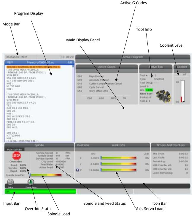
Above is a view of the control panel in Memory Mode with the Program Key active on the Display Key. The Main Display Panel varies according to which of the DISPLAY keys are active.
