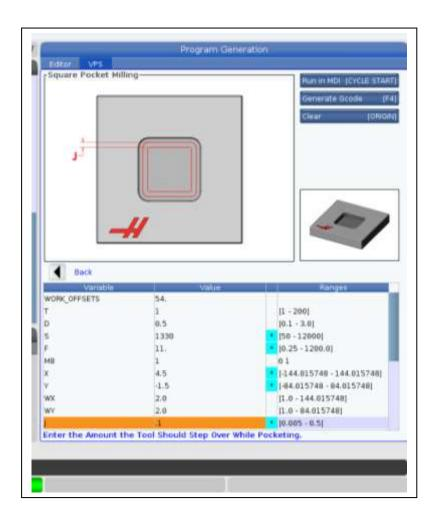
Going back to the VPS directory the square pocket option is highlighted and entered to give the above menu to be filled in. The same feeds and speeds as the circular pocket are entered along with the location of the middle of the pocket and the size of each side. A step over of .1 is entered for the J value.
