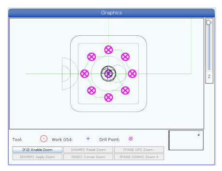
In the graphics mode the tool paths run instantaneously. To see the individual tool paths the program must be run in [SINGLE BLOCK] or [OPTION STOP]. The program must be run step by step. This is done by pressing the [CYCLE START] key repeatedly.
