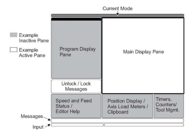
The new 16 software has a larger display and more panes than older versions. Above is the basic display layout. What is displayed depends on which display keys have been used. The only pane active is the one with the white background. Only when a pane is active may changes be made to data.
