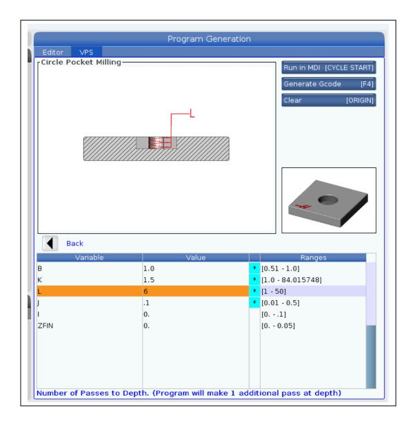
With the VPS a start drill hole is not required. The end mill circular ramps (helical interpolates) down to create a starting hole. The largest diameter an end mill can circular ramp down is 2 times the diameter. For a .5 inch end mill that gives B value of 1. K is the final diameter of 1.5" if the pocket.
