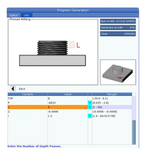
The code for circular pocket milling the minor and thread milling created is using VPS Note with the VPS thread milling the cutting starts at top using G2 (clockwise radius) which is conventional milling. To use climb milling the thread milling starts at the bottom and G3 or counter clockwise radius is thrown going in the positive Z direction.
