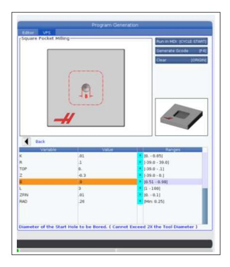
On the second page a finish pass of .01" is inserted for K. Depth information is given for the Z. The square pocket also circular interpolates to give a starting hole similar to the circular pocket. The size is indicated in B. The number of step downs is given in B. Radii will be created in the corners of .26.
