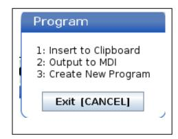
This will put the contour milling code in the clipboard which than can be pasted at the end of the original program using the F4 key.
