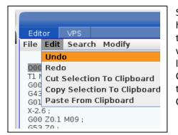
Several lines of code can be selected by using the F2 key. First highlight the first line of code and press F2. Then cursor down to the last line of code that needs to selected and press Enter. This will select several lines of code and they will be highlighted in a light blue. This selected text can be either cut or copied to the Clipboard. From the Clipboard it may be pasted anywhere in the current program of another program using the Paste from Clipboard option.
