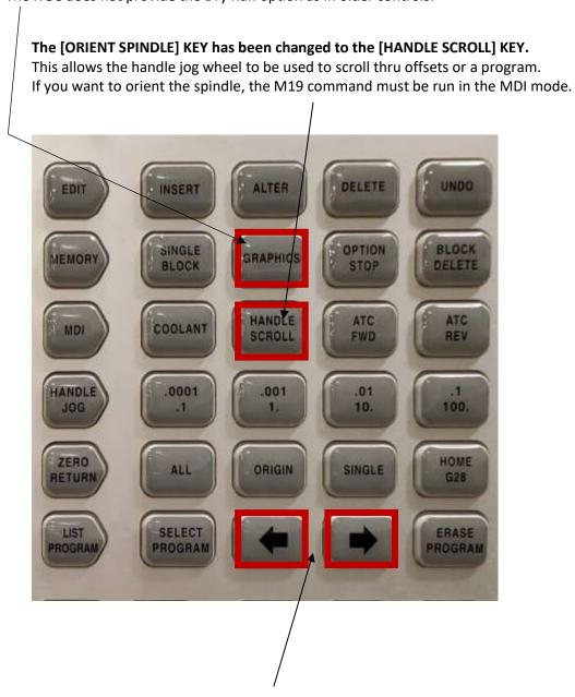
**The [SEND] AND [REC] KEYS have been changed to FORWARD and BACK KEYS.** These keys allow navigation forward and backward thru page history. NGC does not provide for a RS232 port. Only Ethernet connections are available or an upgrade to WIFI.
