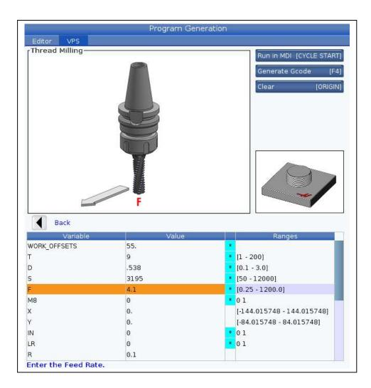
The pitch of the thread must be entered as below. The pitch for 12 threads/in =1/12=.0833.
