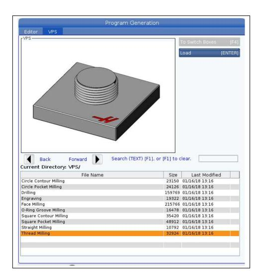
The following example shows using VPS to create the code for a 1.5"-12 internal thread. Thread minor 1.439".
