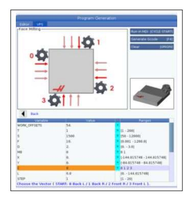
Below the step over width was calculated at 75% of the tool width. Also note R set to .1. Z in work coordinates set to zero. D is set to 1 for only one pass.
