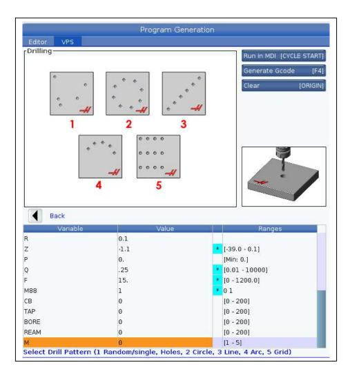
Below information on bolt hole location, radial size, starting angle, and number of holes is indicated.
