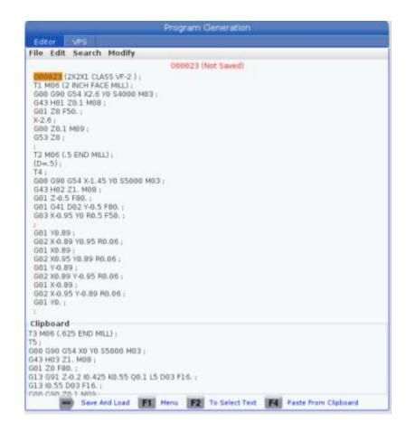
Above is the screen in the edit mode. To edit a word highlight it and then press DELETE, INSERT, ALTER or UNDO keys to change the program. Note on the bottom of the screen the program is not saved until the [MEMORY] key is pressed. Text may be selected to put in the Clipboard by using the [F2] key. [F4] allows you to paste code from the Clipboard to your program.
