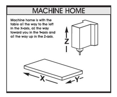
This is crucial to the operation and function of a CNC machine as all of our programs, fixtures, and tooling are based off of the **machine home position described as X0, Y0, Z0**.
