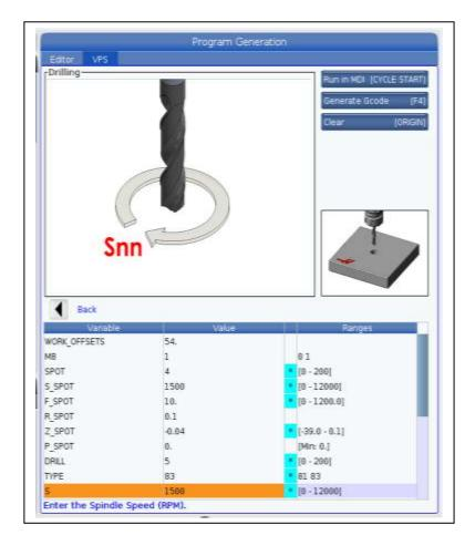
Below the depth, peck length, feed and thru the spindle coolant (M88) are indicated. M gives the different hole placement options that may be used. In option 1 the X and Y locations of all the holes may be given. Option 2 bolt circle with holes equally spaced may be indicated. Option 3 holes equally spaced along an angle may be given. Option 4 bolt hole circles equally spaced by an angle may be created. Option 5 holes along a grid may be given.
